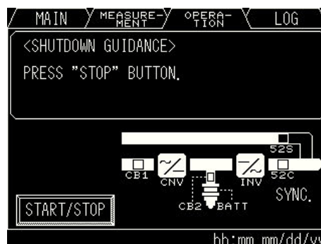
Figure 2.3(c) Shutdown Guidance
